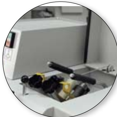
Bandspannung manuell / belt tensioning manually
